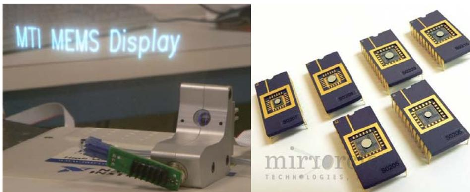
*Figure 1. Mirrorcle MEMS mirror technology. On the left a laser display unit is writing text on a transparent film with special coating. On the right are MTI's various MEMS mirror designs.*
