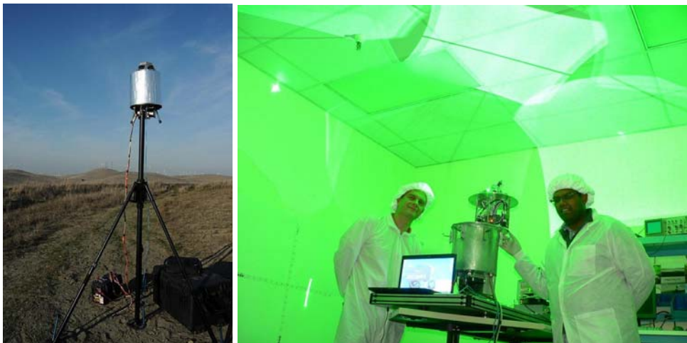
Figure 2. Mirrorcle Hemiscan is photographed in its outdoor tests, fully stand alone and battery powered. To the right is an indoor lab test at Mirrorcle Technologies showing the opened unit and seven laser beams simultaneously scanning above the engineers' heads.
