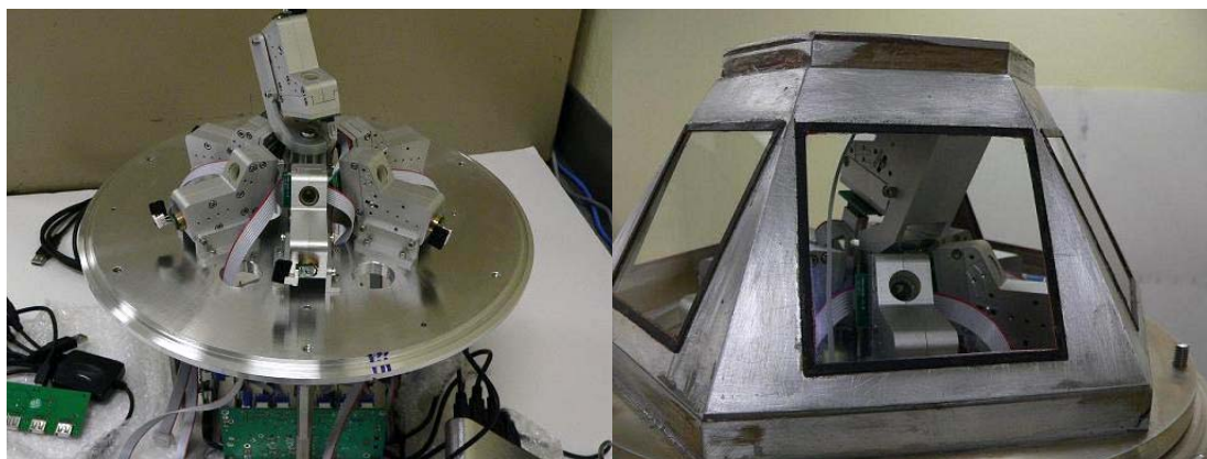
Figure 1. Mirrorcle Hemiscan - Mobile, robust, extreme wide-angle laser scanning system designed for indoor and outdoor use.
