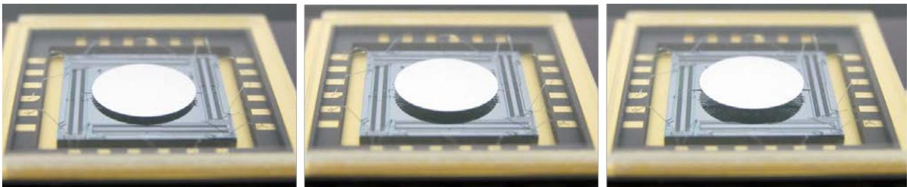
*Figure 1. Mirrorcle's 5.0mm MEMS mirror with A4QQ8.3 actuator chip in DIP24 package actuated in purely pistoning (z-axis or up/down) motion. Middle image is taken at the origin/rest position. Left image at maximum down position of  $\sim -0.1$ mm and the right image at the maximum up position of  $\sim +0.1$ mm.*
