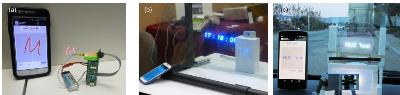
Figure 8. Playzer prototype showing mobile content examples, (a) Displaying a freehand drawing. (b) Displaying current time (c) Smartphone device connected to our virtual image HUD prototype creates and streams text content.
