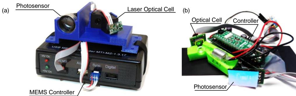
Figure 9. (a) Laser Tracking and MEMS Mirror Demonstrator Kit controller, with the laser optical cell and photosensor, (b) A reduced size, weight, and power consuming version of the MEMS controller with optical cell and photosensor.
