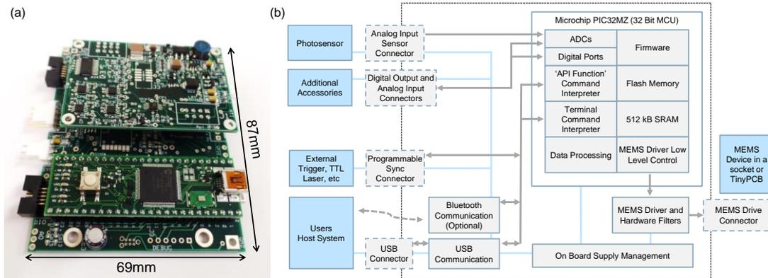
Figure 8. USB-SL MZ MEMS controller: (a) The development kit controller measures 69mm x 87mm, (b) Diagram of controller
