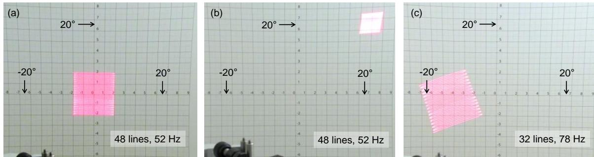
Figure 5. The reference graph shown behind the scan has each unit increment representing 3° optical degrees. (a) Example of a raster scan with 48 lines, scanning at 52 Hz, over a 12° x 12° area, (b) The same resolution of the scan, with 48 lines updating at 52 Hz refresh rate is offset to +20° on X-axis and +20° on Y-axis, and scanning a FoV of +/-6°, (c) An example of a raster scan that is rotated at 20° and offset to -12° on X-axis, and -2° on Y-axis, scanning 32 lines at 78 Hz.
