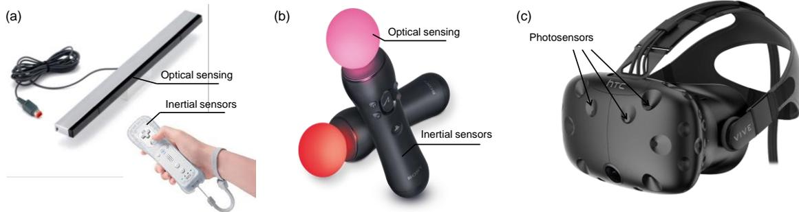
Figure 2. 3D Sensing in gaming and other AR/VR applications: (a)Wii remote and sensor bar to optically track the controller with an inertial sensor, (b) Handheld controllers with built-in inertial and optical sensors (c) VR headsets with photodiodes or retro-reflective markers for position and orientation tracking.
