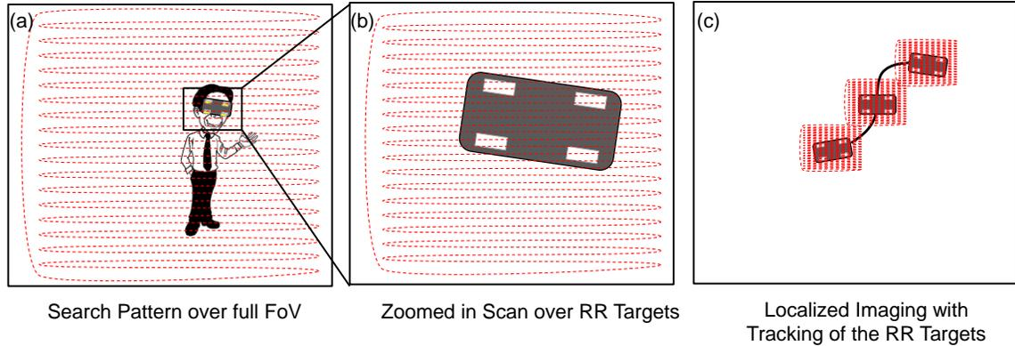
Figure 4. (a) A scan of the full Field of View (FoV) to image and detect any retro-reflective (RR) targets, (b) the same resolution and refresh rate is used to zoom in to the area around the headset with the RR targets, (c) While maintaining the zoomed in scan, the VR headset is tracked by offsetting the position of the scan after each frame – updating the position of the scan at the refresh rate.
