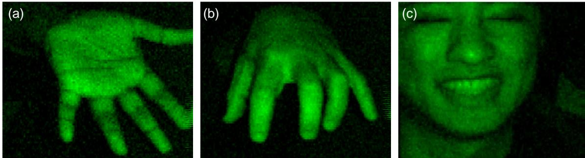
Figure 10. (a) The single-pixel camera imaging a hand ~1m in front, with 60 lines, and 16 Hz refresh rates, (b) Another image of a hand with the same resolution, (c) an image of a face scanned ~1m in front of the imager.
