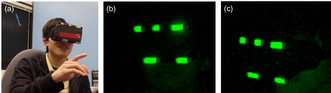
Figure 11. (a) The single-pixel camera raster scanning over the VR headset with retro-reflective markers, (b) a zoomed scan of the 5 RR markers on the VR headset, (c) Another frame of the zoomed scan of the VR Headset with the head tilted and rotated to a different position. The location of the constellation of RR markers can be used to determine 3D orientation and position of the VR Headset.
