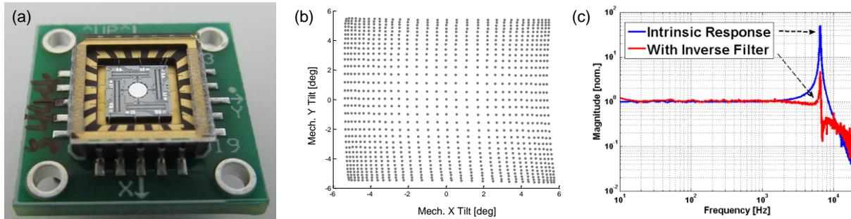
Figure 6. MEMS Mirror Device used in this work: (a) Photograph of the A3112.2 MEMS device packaged in a 9mm wide ceramic carrier, (b) 2D look-up table (LUT) of the X and Y mechanical tilt recorded on a PSD. The optical distortions seen on the LUT are due to  $22.5^\circ$  angle of incidence of the scanning laser on the MEMS device. (c) Intrinsic frequency response of a device with a 6200Hz resonance and frequency response of the device with inverse filtering applied.
