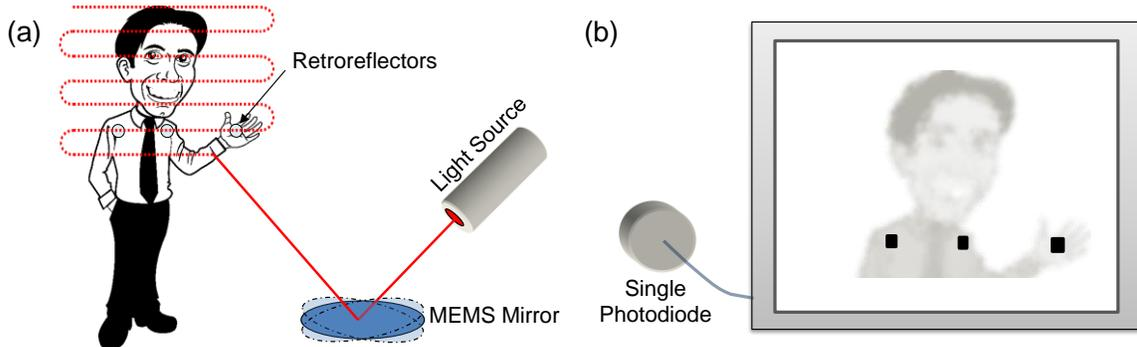
Figure 3. Testing setup for position tracking: (a) A MEMS mirror steers a light source in a raster pattern across the field of regard, (b) A single photodiode measured the returned light at each point and displays the reflected intensity on a screen.
