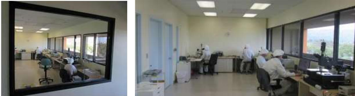
Figure 2. Mirrorcle's new "White Lab" cleanroom with die-attach equipment, wire-bonder, probe station, optical QA capability and storage stations. Over 1600 square feet of MTI's new facility are Class 10,000 or better cleanroom, with 8 HEPA filters ensuring dust-free air.
