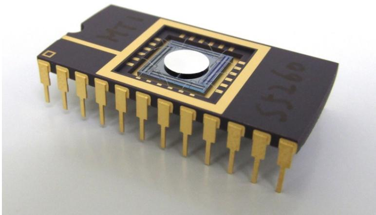
*Figure 1. Mirrorcle's first-ever 5.0mm MEMS mirror with A4SR8.3 actuator chip in DIP24 package. This device offers an angular reach of 5 degrees at 500Hz fres.*
