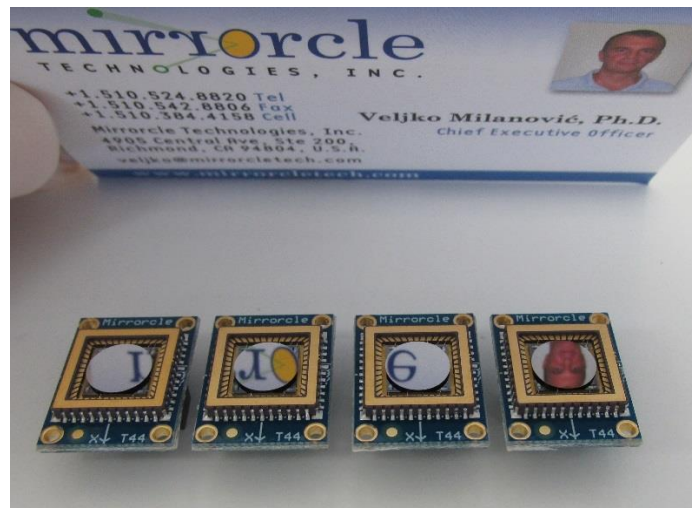
Figure 1. Mirrorcle's 7.5mm Al-coated MEMS mirrors with A5L2.1 actuator chips in TINY48.4 connectorized packages. These devices offer a total angular reach of \sim 2.0 degrees mechanical in both X and Y axes.
